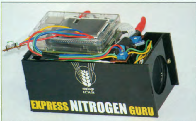
A gadget to detect Nitrogen deficiency in leaves
